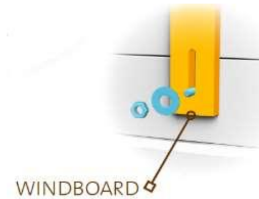
14. Windboards with bolts
